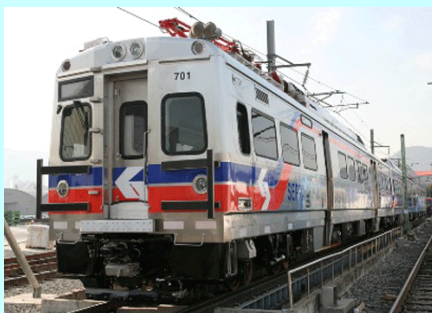
Southeastern Pennsylvania Transportation Authority [SEPTA] sidelined all 120 of its Hyundai Rotem electric multiple-unit coaches after suspension problems were discovered July 1, Philadelphia media outlets reported. Cracks were found in the equalizer beams in the truck assemblies. With one-third of its Regional Rail fleet out of action, SEPTA leased locomotives and coaches from Amtrak and NJ Transit and coaches from Maryland MARC. The cost to lease equipment will top $257,000 per month and regular service is not expected to return until after Labor Day, The Philadelphia Inquirer reported July 11. In the interim, SEPTA has put into effect a modified weekday schedule on 12 routes with the Cynwyd shuttle replaced by buses. Rail service now is handled by GE Silverliner IV cars built in 1971 augmented by the leased rolling stock.
